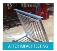
A 30 kg sand bag impact test was performed on the NewYork balustrade as shown above. As per the engineer, the impact test was successful as the sand bag did not pass through the balustrade.
